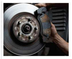
insist on new components to ensure the pads can move freely in the bracket but not have excessive play. If you replace rotors, don't purchase the cheapest ones you can find – because inexpensive rotors can actually move and flex. While not visible to the naked eye, this movement can cause noise. The same goes for the brake calipers – Quality heavy calipers will dampen vibration and keep a consistent "friction footprint" between the pads and the rotor's face under different braking conditions.
